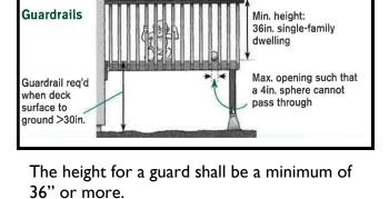
All openings on a guard/railing shall not allow for the passage of a 4" sphere.
